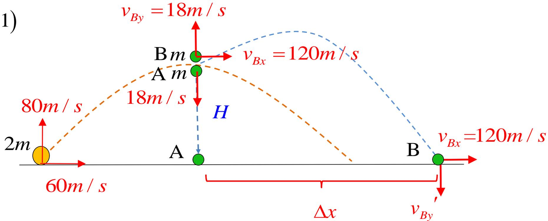
原物體自拋出到最高點： $\left[ H = \frac{v_0^2}{2g} \right] H = \frac{80^2}{2 \times 10} = 320 [m]$
