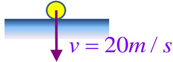
$$\vec{J}_{\text{合力}} = (\Delta \vec{P}) = m \Delta \vec{v} = 2 \times (0 - 20) = -40 [\text{kg} \cdot \text{m} / \text{s}]$$
