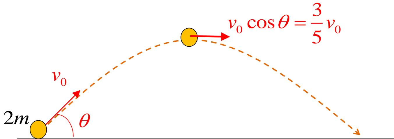
$$v_0 \cos \theta = \frac{3}{5} v_0 \rightarrow \theta = 53^\circ$$
