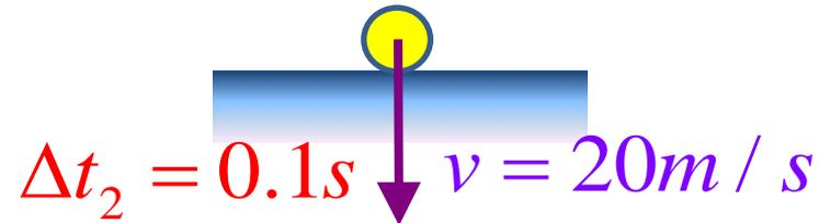
$$\vec{F}_{\text{合力}} = \left( \frac{\Delta \vec{P}}{\Delta t} \right) = \frac{m \Delta \vec{v}}{\Delta t_2} = \frac{-40}{0.1} = -400 [N]$$
