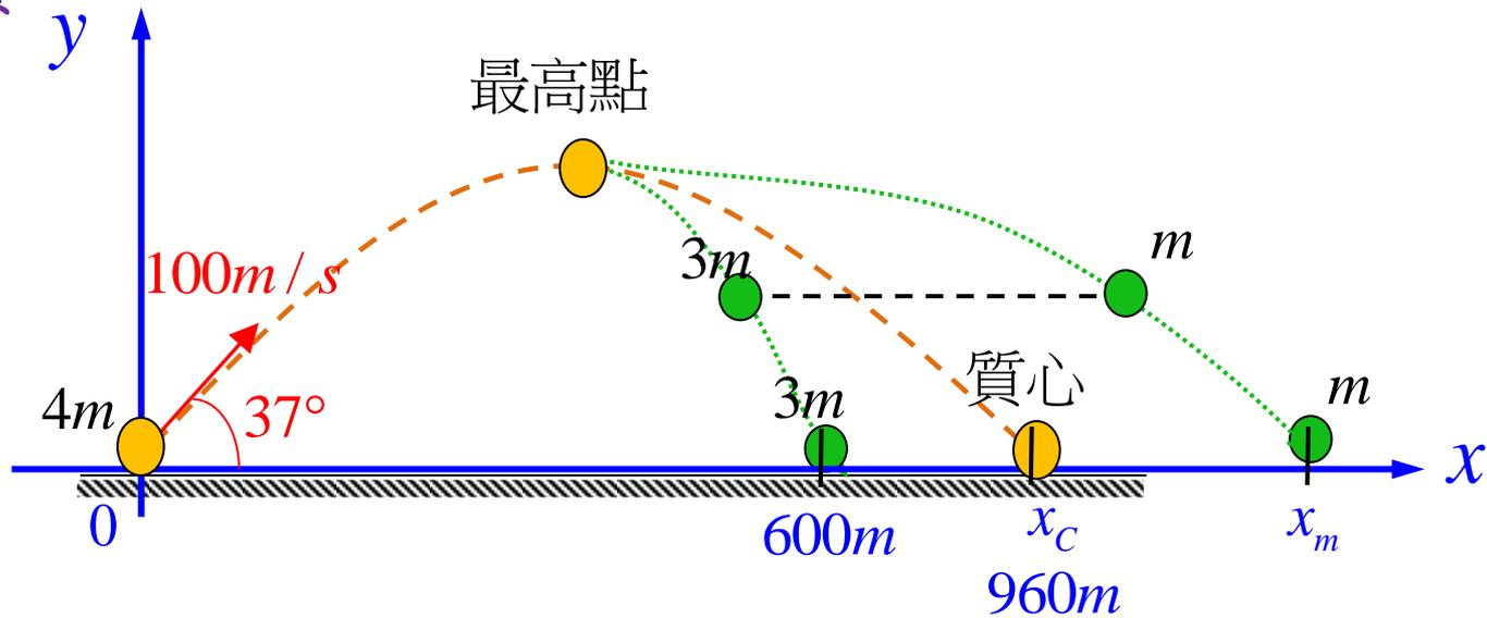
$$\left[ R = \frac{2v_0^2 \sin \theta \cos \theta}{g} \right] \quad x_c = \frac{2 \times 100^2 \times \frac{4}{5} \times \frac{3}{5}}{10} = 960 [m]$$
