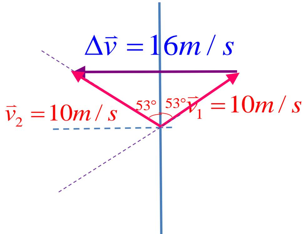
$$\Delta \vec{P} = m \Delta \vec{v} = 5 \times 16 = 80 [kg \cdot m / s] \text{ 向左}$$
